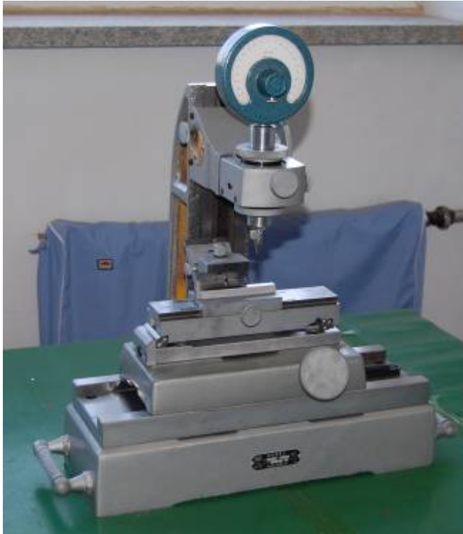
Measuring Instrument of Ring angle
