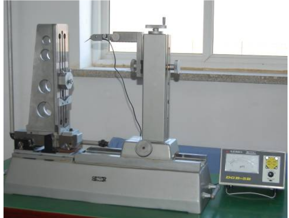
Measuring Instrument of diameter, angle and linearity for taper Rollers
